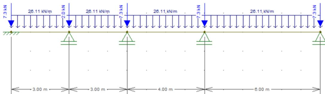
**Figura 22 – Cargas sobre as vigas**
